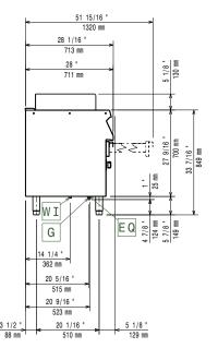
EQ = Equipotential screwG = Gas connection
